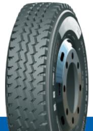
©The design of three tortuous V-shaped large-angle grooves makes it have good maneuverability.
