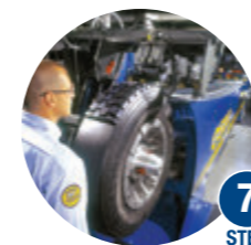
7 STEP Precured tread application process
